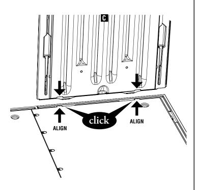
Hold Repeat Left Side (C) upright to prevent it from falling (until Left Back (D) is installed).
